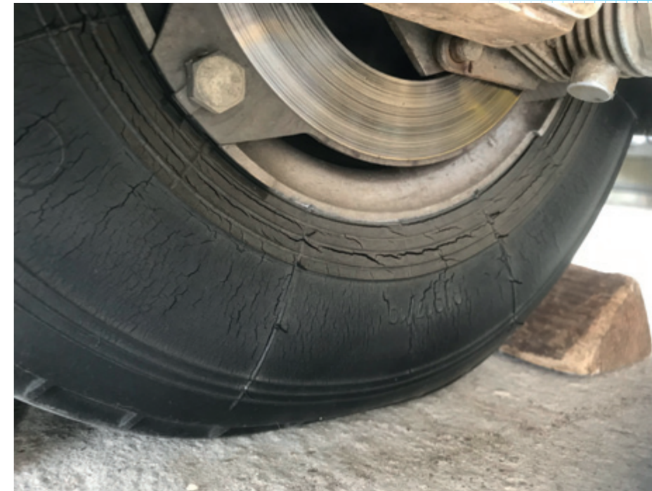
If the sidewalls are cracked, the tyre needs replacing
