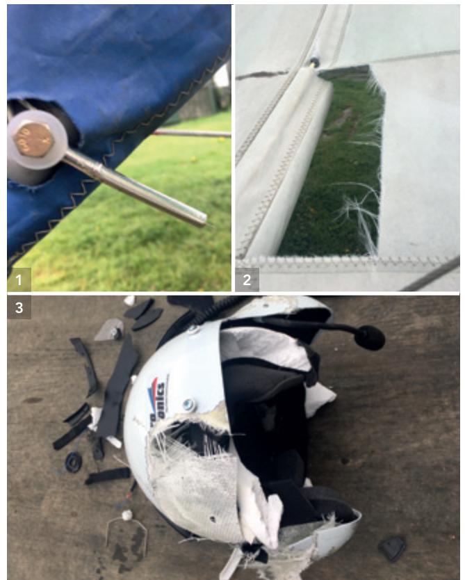
(1) Broken cable end; (2) damaged wing fabric; and (3) the offending helmet – thankfully without a head in it
