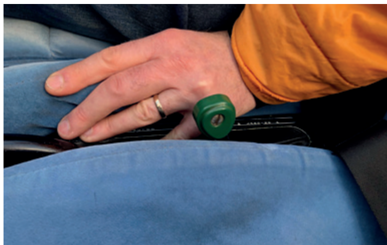
Eurostar (from top) Fig 1 Trim operated via a lever between the seats Fig 2 Easy for a passenger to accidentally catch the lever Fig 3 A misplaced hand may have been the cause of two fatal accidents
