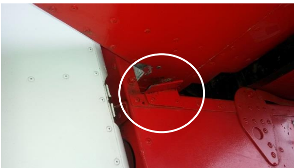
Figure 3.1 - elevator 'down' stop
