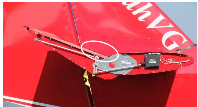
Figure 3.2 - elevator 'up' stop
