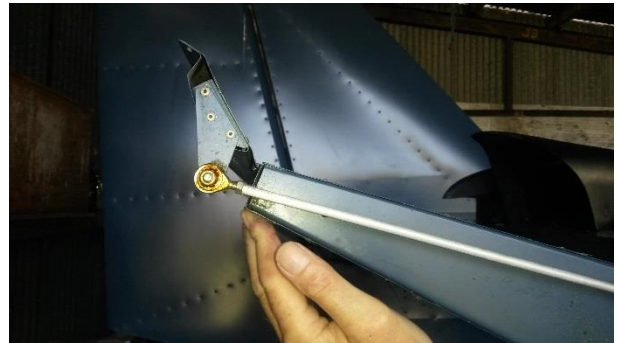
Figure 8.2: trim tab in no danger of going 'over-centre' (compare with fig 6.1)
