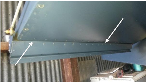
Figure 8.1: positive clearance between trim tab and elevator
