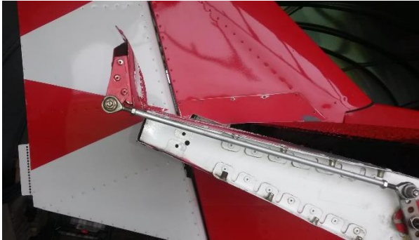
Figure 6.1 - incorrect (small) horn from obsolete bungee trim system
