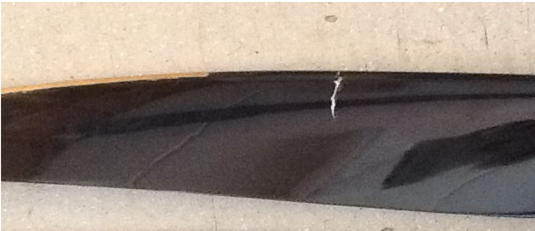
Figure 1 – transverse crack Kievprop on propeller blade
