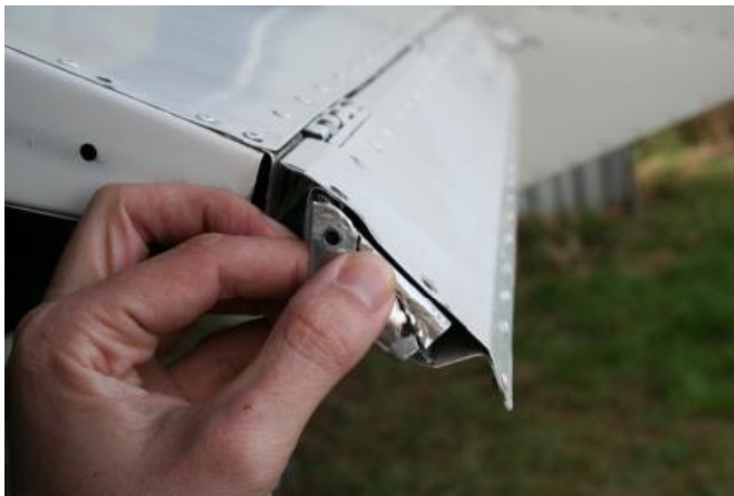
Figure 2: Fractured end ‘closure’ rib held in original position in port end of port anti-balance tab. The rivets attaching the control horn in place on the end ‘closure’ rib, and the rivets attaching the end ‘closure’ rib to the anti-balance tab, were drilled out subsequent to the in-flight failure.
