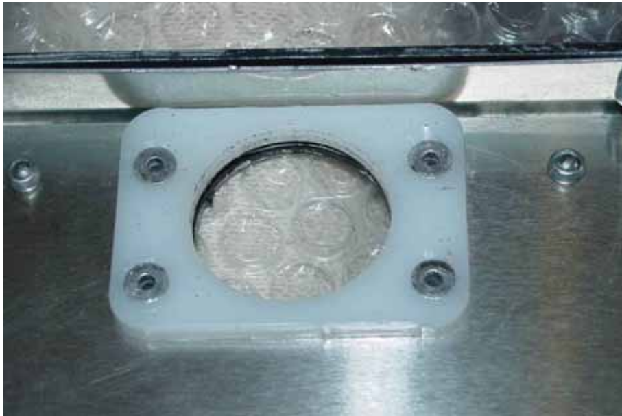
Figure 5 – View looking at forward face of cross-member with nylon bush reinstalled
