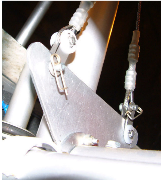
Figure 4; aileron cable connections viewed from beneath.
