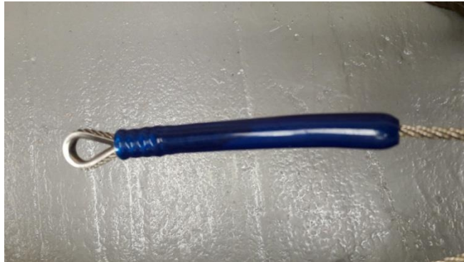
Fig 3. A thimble and Nicopress sleeve type fitting. The blue plastic shroud can be pulled back for inspection of the sleeve.
