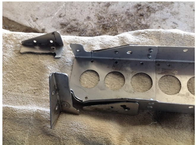
Figure 2.2: cracked bracket after having been removed from aeroplane
