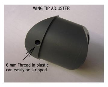
Owners have been known to over tighten the socket head screw in the tip adjusters, check that the screw is present and tight. Note NO washer should be fitted here, the tip adjustment depends on the socket head screw biting directly into the leading edge.
