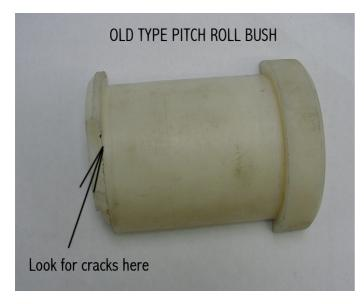
The original tolerance in the roll bush was increased to stop roll stiffness if the bush should swell. Following the tolerance change a few roll bush flanges were found to have cracked and/or broken away. The flange length was therefore increased as shown in the photo below. On early wings check carefully for cracking.
