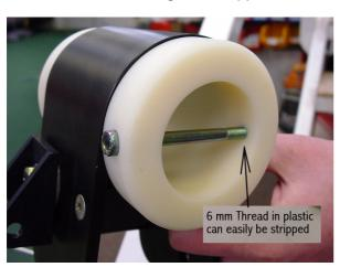
Check socket screw for tightness and stripped threads. Do not over tighten, as the tube will be distorted causing the roll bearing to become stiff.
