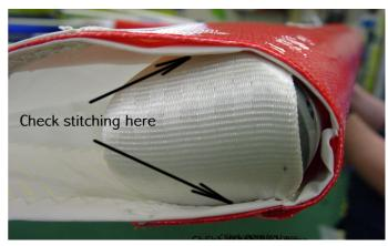
It is vital that all wings have had service bulletin 84 carried out. Where the tip modification has not been carried out the UV/abrasion protection patch must be glued properly in place and no broken stitches holding
