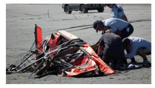
**OUTCOME:** Crash resulted, due to crack in seal giving lean mixture & low compression on 2 cylinders
