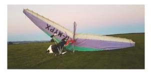
'When the microlight was about 30 feet above the runway it rolled "violently" to the right in the wake of the twin that had just landed, and hit the ground in a nose-down attitude
