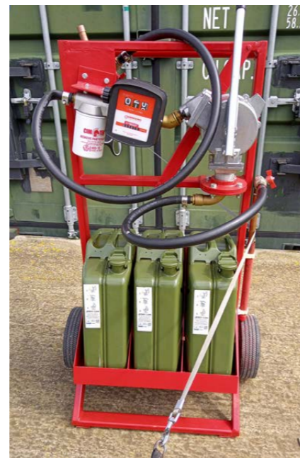
Paul Ellis' fuelling system delivers up to 110 l/min
