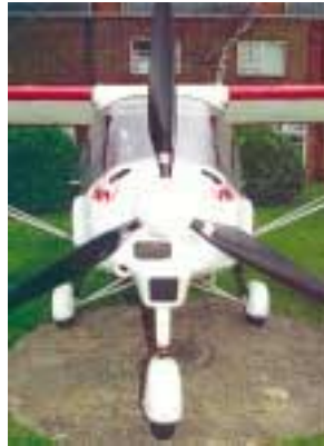
Latest UK 912S Aircraft uses Arplast Prop. Warp drive on this earlier example.
